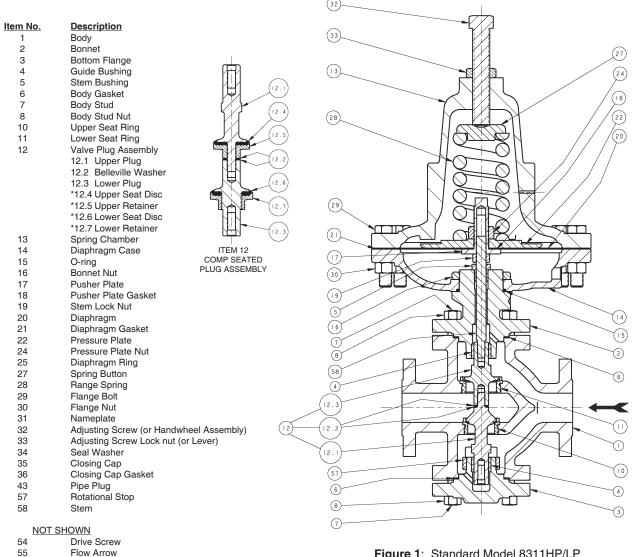
Figure 1: Standard Model 8311HP/LP (NOTE: Variation "LP" has a larger diaphragm area than the "HP".)
